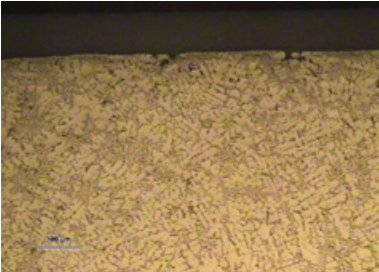
Photo 10. Micrography EN AC 46200 Magnification 500x
